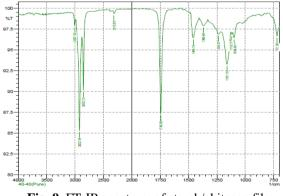
Fig. 9. FT-IR spectrum of starch/chitosan film
