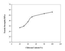
Fig. 2. Effect of chitosan on tensile strength of starch-based film
