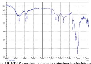
Fig. 10. FT-IR spectrum of acacia catechu/starch/chitosan film
