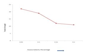
Fig. 4. Effect of Acacia Catechu on tensile strength of starch-chitosan based films
