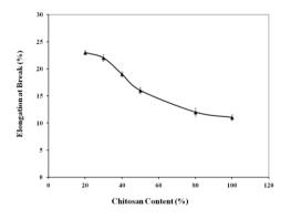
Fig. 3. Effect of chitosan on elongation at break of starch-based film
