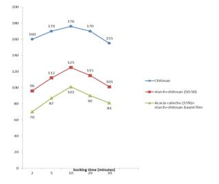
**Fig. 12**. Water uptake of pure chitosan film, chitoan/starch film and acacia catechu (0.15%) + starch + chitosan film
