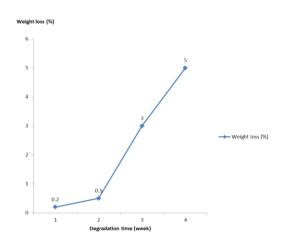
**Fig. 13.** Soil degradation of chitosan/starch based film with acacia catechu (0.15%)
