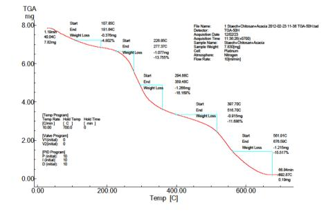
Fig. 6. Thermo-gravimetric analysis of starch + chitosan + acacia catechu film
