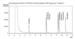
Fig. 3. Chromatograms of standards of organophosphorus insecticides run by GC-FTD
