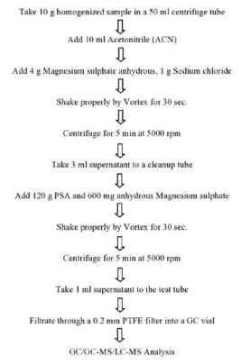
**Fig. 2.** The flowchart of extraction of pesticide by modified QuEchERS method
