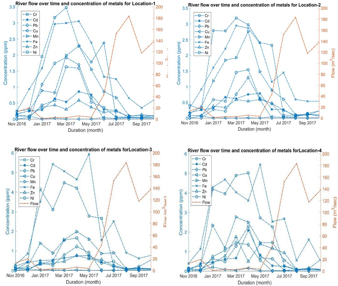
**Fig. 2.** Impact of river flow on chromium, cadmium, lead, copper, manganese, iron, zinc and nickel concentrations of four sites both in low flow (Jan-May) and high flow (Jun-Oct) seasons.
