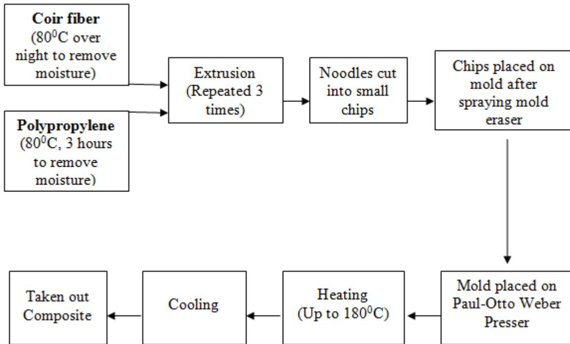
Fig. 1. Flow diagram process of coir fiber reinforced polypropylene composite.
