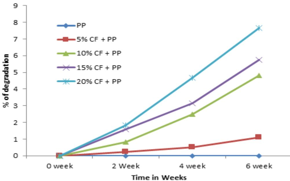
Fig. 2. Degradation of CF+PP composites in soil.
