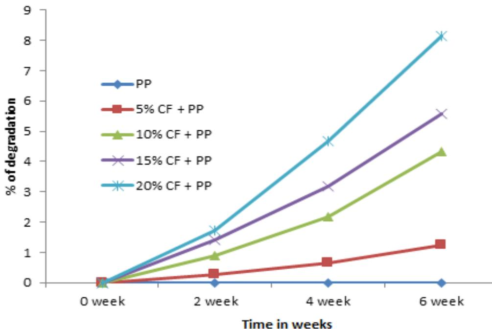
Fig. 3. Degradation of CF+PP composites in saline water.
