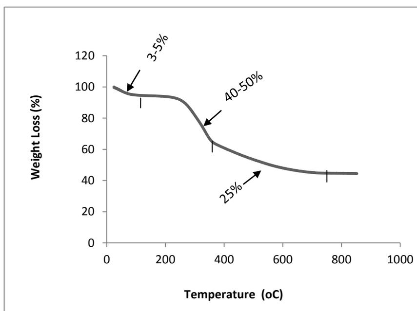
Fig. 1. Thermo gravimetric (TG) curves of RH
