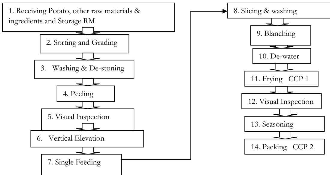
Figure-2: Process flow diagram of Potato Chips
