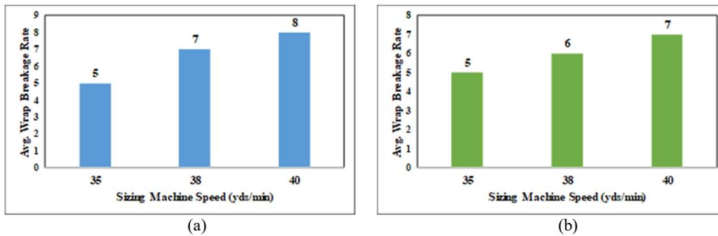
**Figure 2:** Various sizing machine speed and their impact on the average warp breakage rate (a) for shift A and (b) for shift C.
