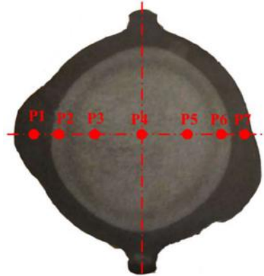
Figure 3: Hardness measurement location identification.
