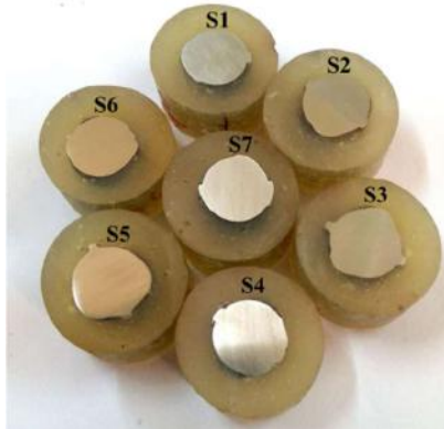
Figure 2: Cold mounted samples after coarse polishing
