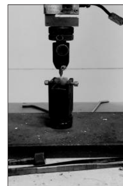
Figure 3 Fracture resistance test by universal testing machine
