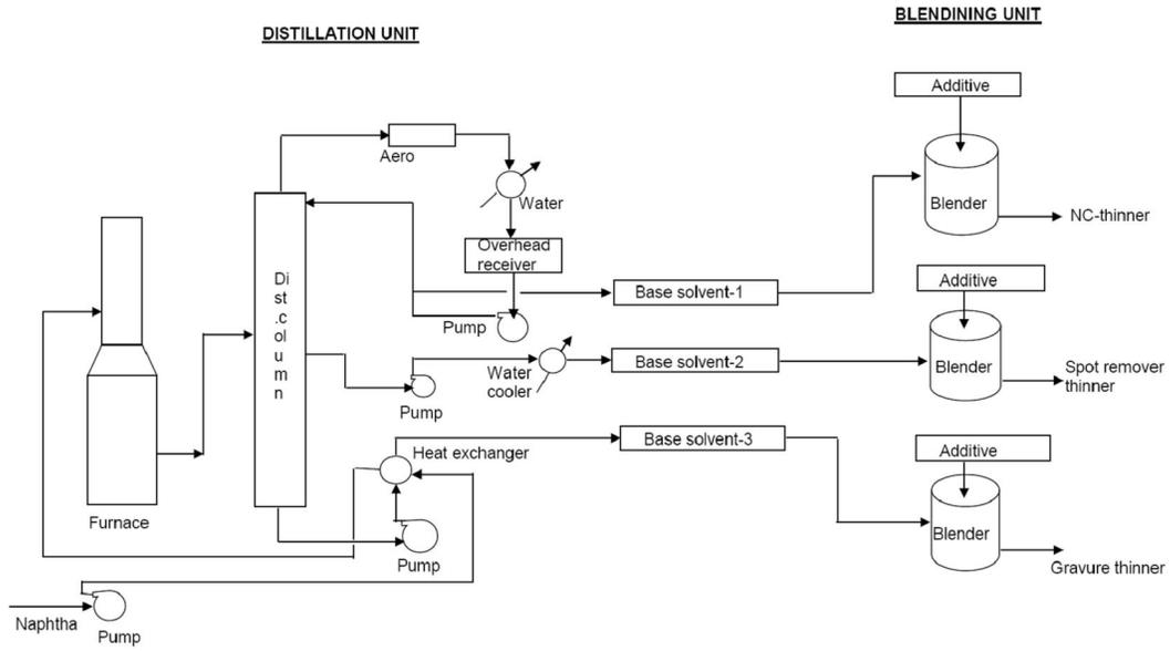
Fig 1. Schematic diagram of a condensate fractionation plant
