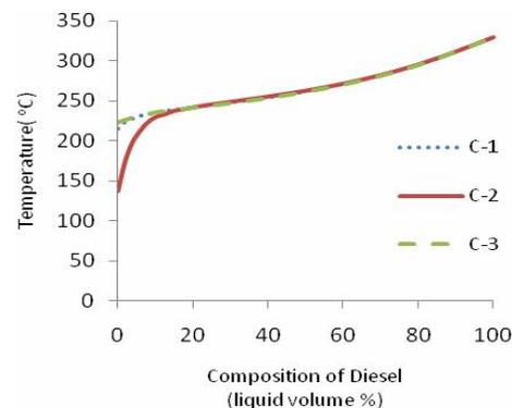
**Fig 3(c).** ASTM D86 data for Diesel obtained from the three different design consideration
