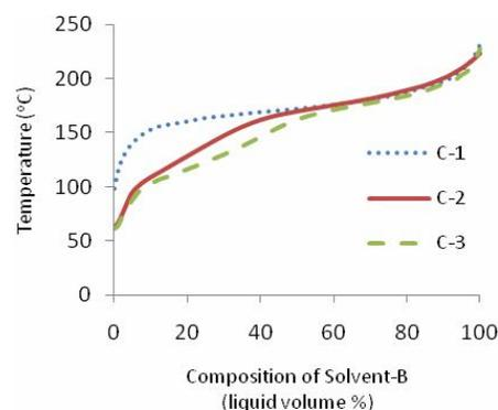
**Fig 3(b).** ASTM D86 data for Solvent-B obtained from the three different design consideration
