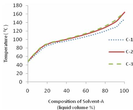
**Fig 3(a).** ASTM D86 data for Solvent-A obtained from the three different design consideration
