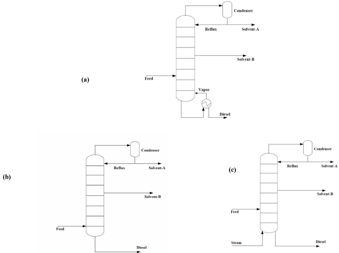
Fig 2. Design variations of the fractionation column – (a) Column-1, (b) Column-2, (c) Column-3
