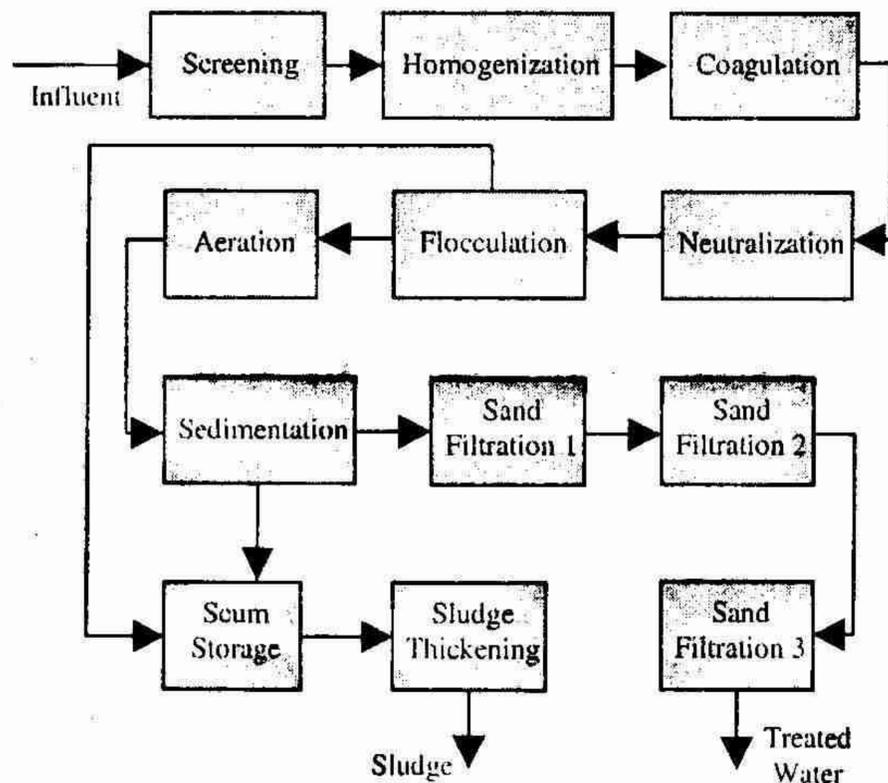
**Fig. 1: Block diagram of wastewater treatment process**
