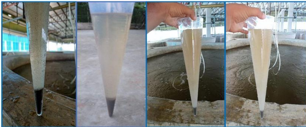
Fig. 4: Measurement of floc using Imhoff cone measurement during experiment.
