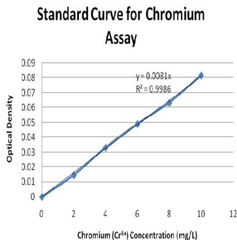
Fig. 2. Standard curve for determination of Cr<sup>6+</sup> reduction
