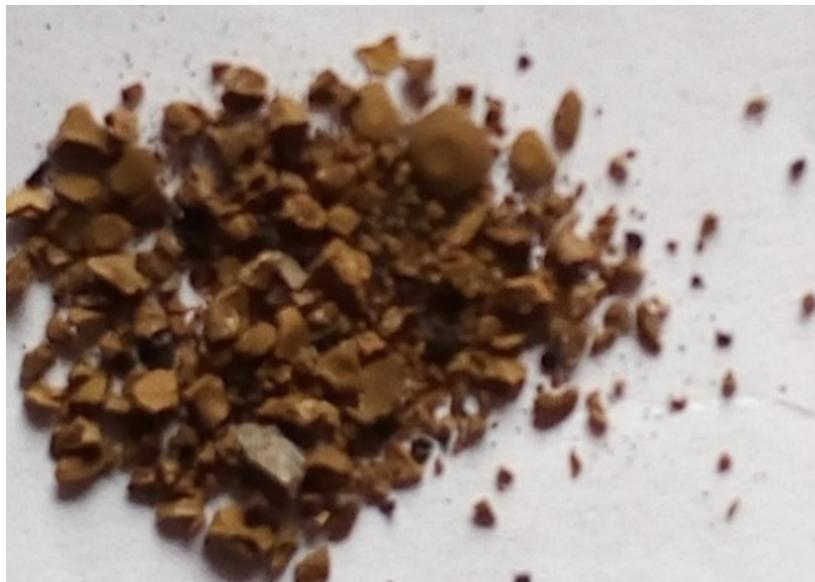
**Fig. 2.** MgO nanorods after calcination at 200 °C.
