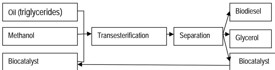
**Fig. 5.** Transesterification by using lipase as catalyst.
