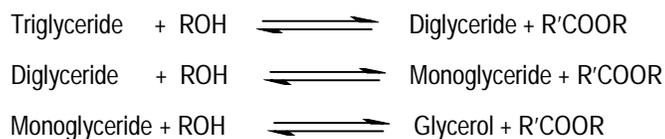
**Fig. 3:** General equations for transesterification on triglyceride.
