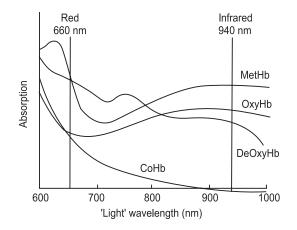
**Fig.-1:** Absorption spactra of normal adult haemoglobin in saturated (OXyHb) and desaturated (DeXoyHb) states, carboxyhaemoglobin (COHb)(, and methaemoglobin (MetHb)
