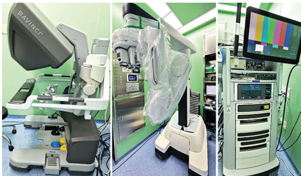
Figure 1: Da Vinci Sp Surgical System- (left to right) A. Surgeon's Console, B. Patient's-side cart, C. Vision Cart (Image: Dr Jhinuk, Korea University Anam Hospital)
