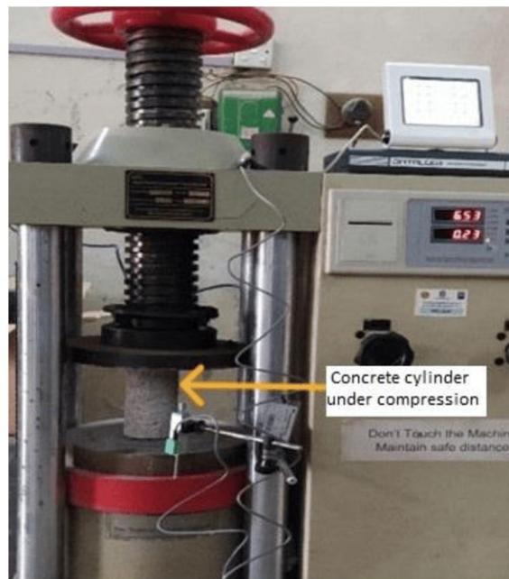
Figure 3: Test setup for compressive strength
