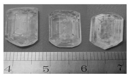
Fig. 3. Single crystals of ZnSO<sub>4</sub>.7H<sub>2</sub>O.
