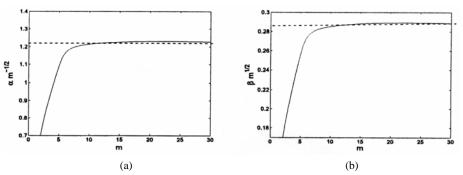
Fig. 1. Magnetic field m versus (a)  $\alpha m^{-1/2}$  and (b)  $\beta m^{1/2}$  for fixed Reynolds number R = 1000. The long curves show numerical results and doted lines show asymptotic ones.
