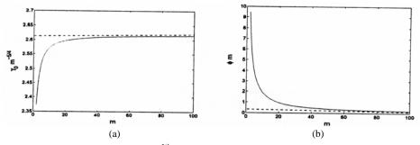
Fig. 2. Magnetic field *m* versus (a)  $\gamma_0 m^{-5/4}$ , and (b)  $\phi m$  for fixed Reynolds number R = 1000. The long curves show numerical results and doted lines show asymptotic ones.
