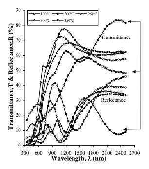
Fig. 3. Dependence of optical transmittance and reflectance on photon wavelength for AGS thin films having different temperatures.
