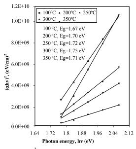
Fig. 4. Variation of  $(\alpha hv)^2$  vs photon energy extracted from absorption coefficient.
