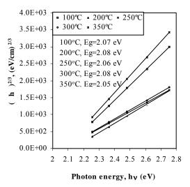
Fig. 5. Variation of  $(\alpha h v)^{2/3}$  vs photon energy extracted from absorption coefficient.
