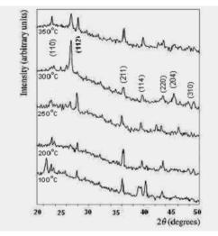
Fig. 1. The XRD spectra of AGS thin films having different temperatures of deposition.
