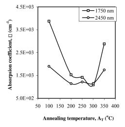
Fig. 6. Dependence of absorption coefficient on temperature for AGS thin films at wavelengths 1750 and 2450 nm.
