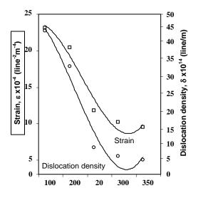
Fig. 2. Dependence of strain and dislocation density of AGS thin films having different temperatures.
