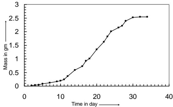
Fig. 2. Mass growth rate of  $\text{ZnSO}_4$  crystal.
