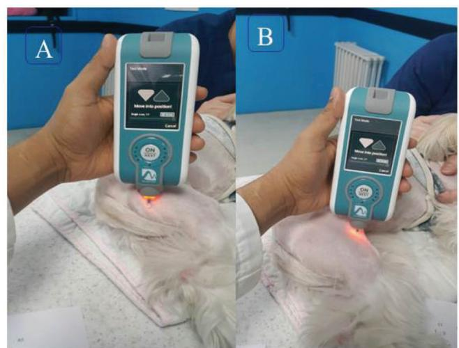
**Figure 3.** Muscle tonicity in the hind limb measured by the MyotonPRO technique. A: measurement of muscle tone from the hamstring muscle; B: measurement of muscle tone from the quadriceps muscle.
