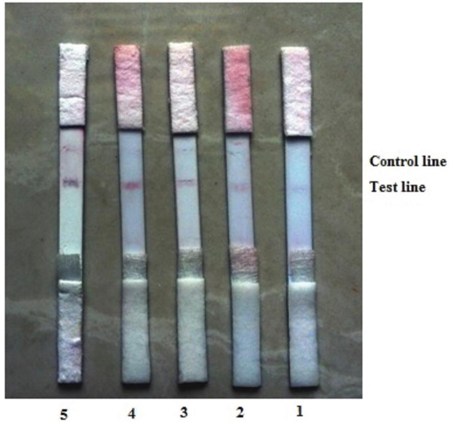
**Figure 9.** Photographs of immunochromatography strip tests performed by adding coffee samples to AA at ratios of (coffee:AA) 0:4 (5), 1:3 (4), 2:2 (3), 3:1 (2), and 4:0 (1).
