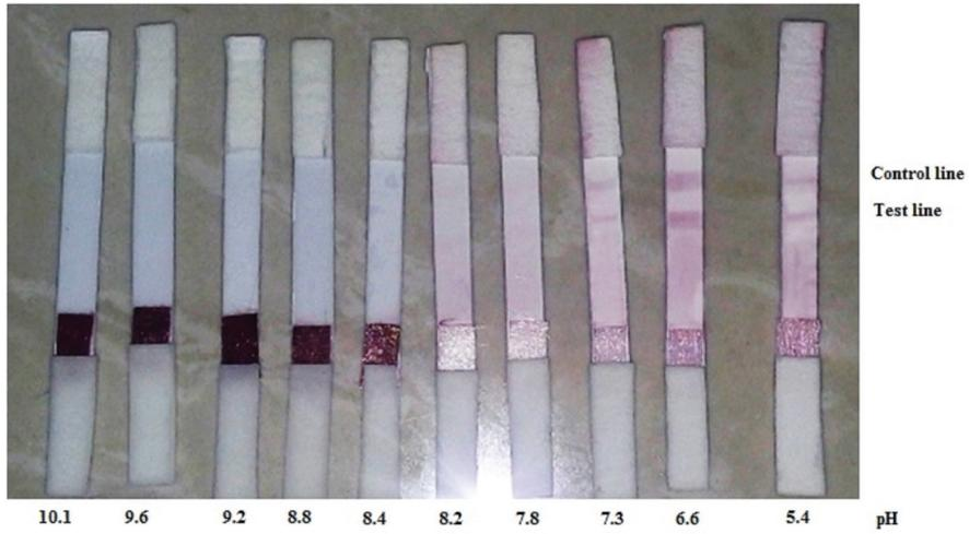
**Figure 8.** Photographs of immunochromatography strip tests for detecting AA using AuNP–Anti-AA antibody conjugates at various pH values.
