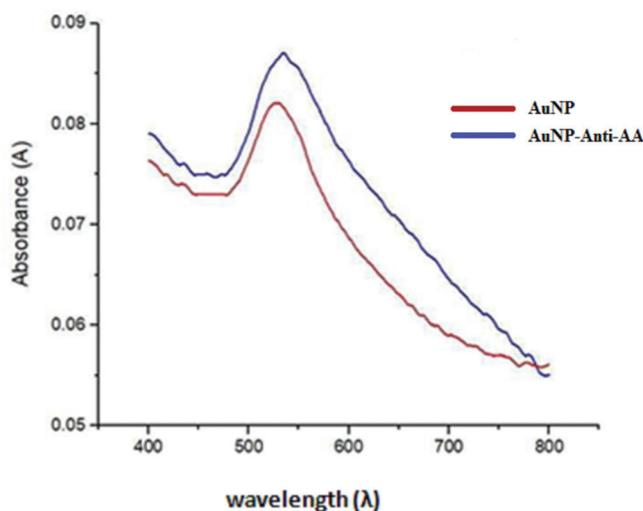
**Figure 5.** UV-Vis Spectra of AuNP in the absence (red line) and presence of anti-AA (blue line).
