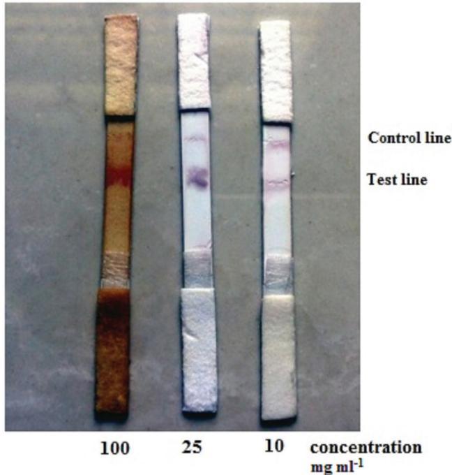
**Figure 10.** Photographs of immunochromatography strip test with coffee samples at various concentrations.
