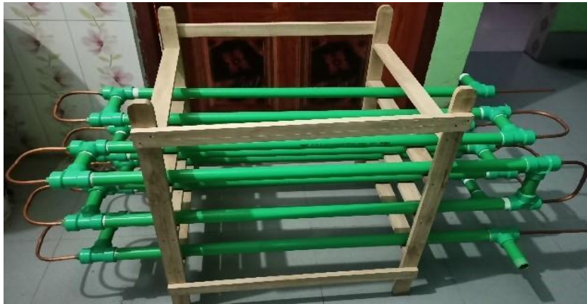
Figure 4: Modified double pipe heat exchanger (Condenser).
