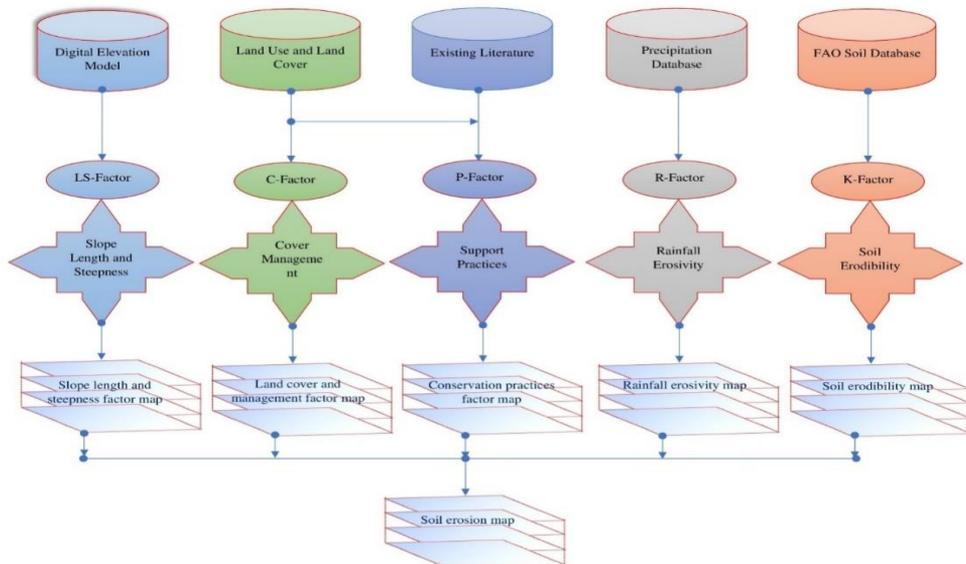
**Figure 2:** The methodological flowchart employed for estimating soil erosion used the RUSLE model
