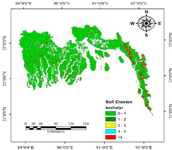
**Figure 4:** Construction of a potential soil erosion map using ArcGIS v. 10.5 and the RUSLE model.
