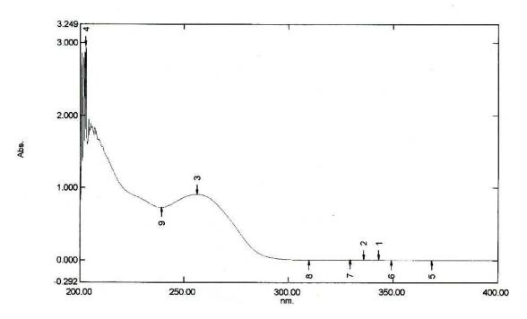
Figure 2: UV spectrum of Olmesartan medoxomil in methanol
