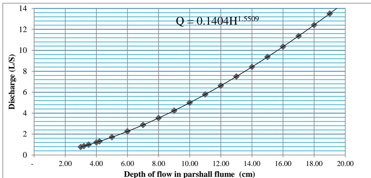
Fig. 2. Head Discharge Relationship of 3 inch parshall flume.
