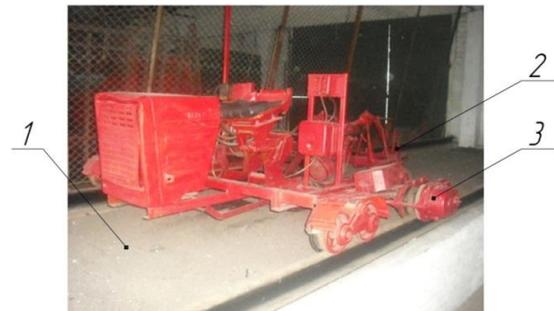
Fig. 2. General view of the sand test bed: 1 - soil, 2 - the coupling device of the discs, 3 - traction transfer device
