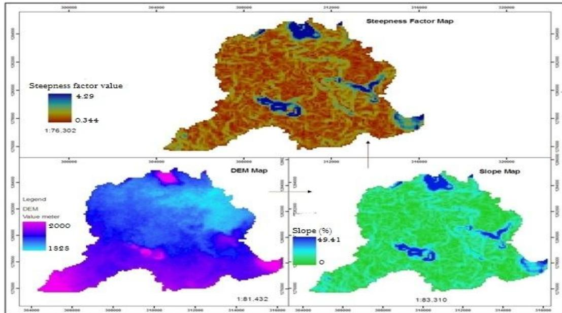
Fig. 6. Derivation of steepness factor from slope map
