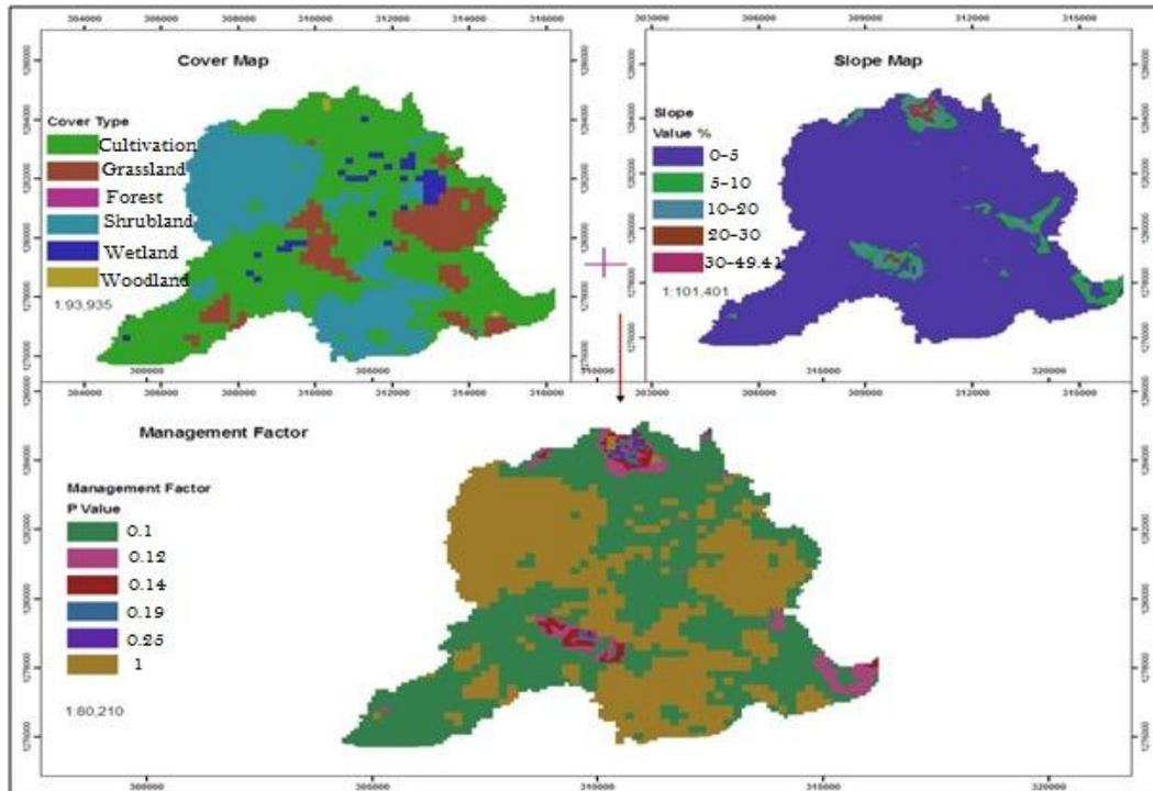
Fig. 8. Derivative of management factor from land cover and slope
