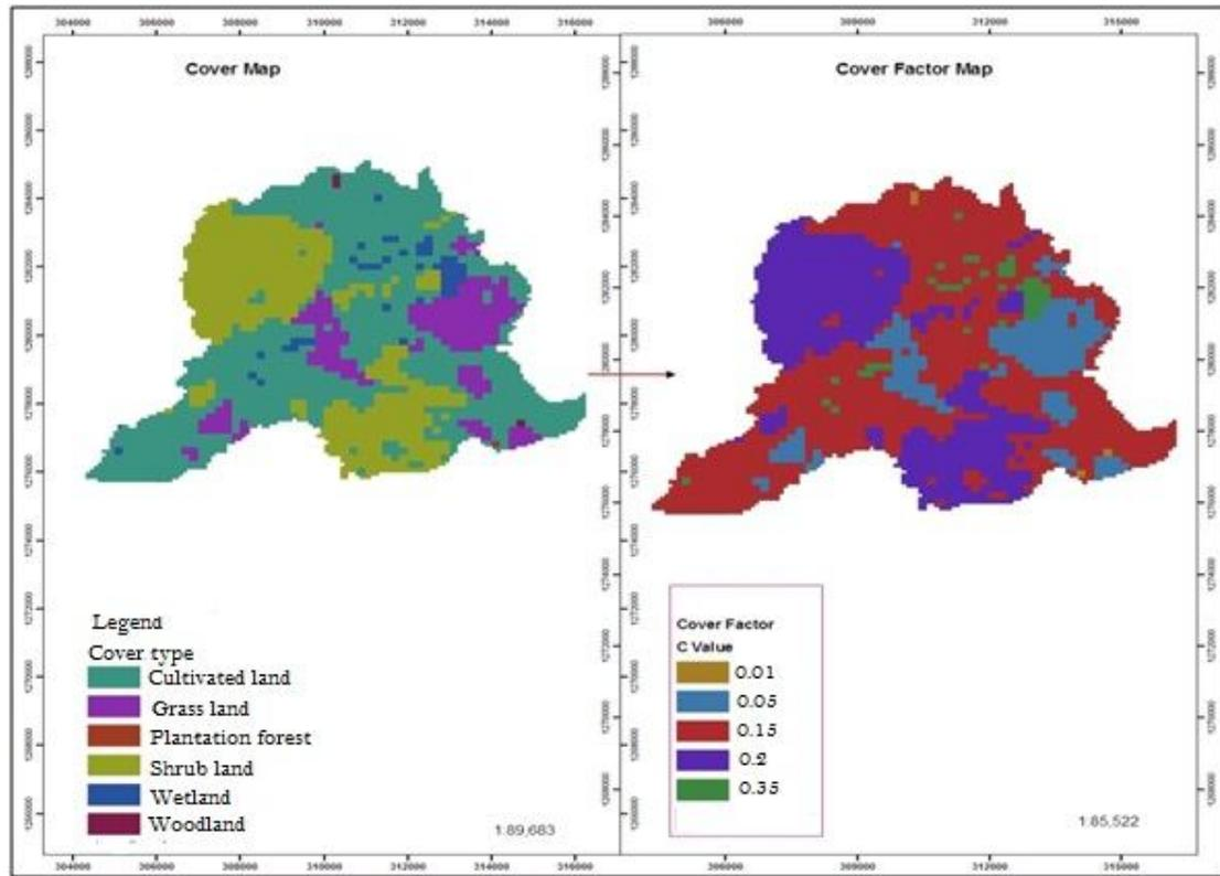
Fig. 7. Derivation of cover factor from cover type
