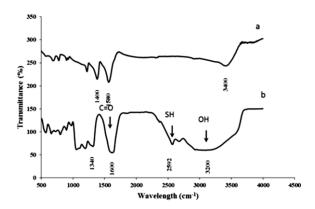
Figure 5: the FT-IR spectra of TGA capped (a) and free TGA (b) CdS nanoparticles.
