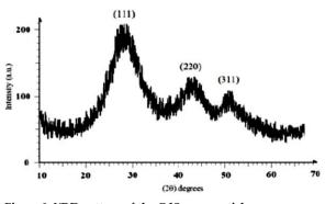
Figure 2: XRD pattern of the CdS nanoparticles.
