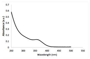
Figure 4: UV-Visible absorption spectra for CdS nanoparticles.
