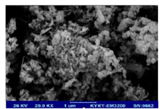
Figure 3: SEM image of CdS nanoparticles.
