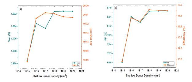
Fig.5. Shallow donor density variation of buffer layer (a) Voc, Jsc; (b) FF, Efficiency
