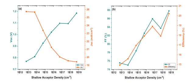
Fig.4. Shallow acceptor density variation of absorber layer (a) V0c, Jsc; (b) FF, Efficiency
