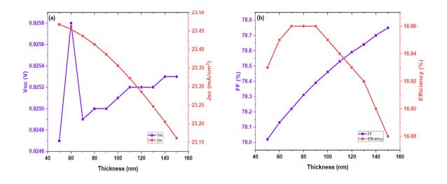
Fig.3. Buffer layer thickness variation (a)Voc, Jsc; (b) FF, Efficiency
