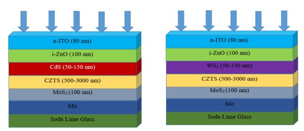
Fig. 1. Device structure of CZTS/WS2 solar cell (a) conventional structure (b) Proposed structure.
