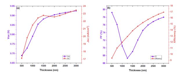
Fig.2 Absorber layer thickness variation (a) Voc, Jsc; (b) FF, Efficiency.
