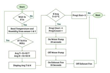
Fig. 6. Flow-chart of proposed system of [20]
