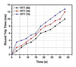
Fig. 8: Round-Trip Delay Comparison with respect to 15, 30 and 50 Nodes
