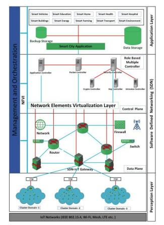
Fig. 4: Proposed "SDoT-NFV" Architecture.
