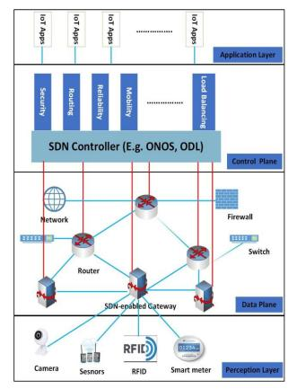
Fig. 2: SDN-IoT Architecture
