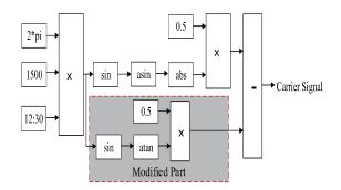
Fig. 4. Modified carrier signal generation for multicarrier PWM technique.
