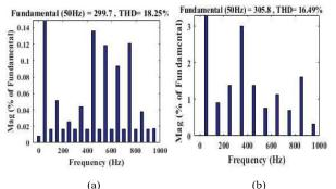
Fig. 9. THD spectrum of Output voltage of cascaded seven level inverter using (a) conventional carrier APOD (b) modified carrier APOD.
