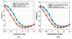
Fig. 12. THD comparison for (a) cascaded seven level inverter (b) reduced switch seven level inverter.
