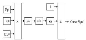
Fig. 2. Conventional carrier signal generation for multicarrier PWM technique.
