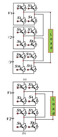
Fig. 1. Seven level inverters (a) cascaded H-bridge (b) reduced switch topology.
