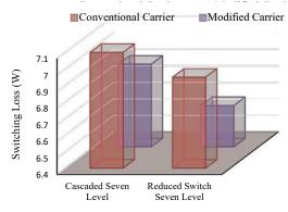
Fig. 13. Switching loss comparison for (a) cascaded seven level inverter (b) reduced switch seven level inverter.
