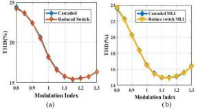
Fig. 11. Calculated THD for (a) conventional carrier APOD (b) modified carrier APOD.
