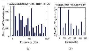
Fig. 10. THD spectrum of Output voltage of reduced switch seven level inverter using (a) conventional carrier APOD (b) modified carrier APOD.
