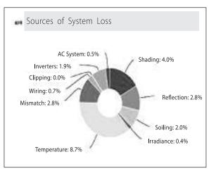
Fig. 3. Sources of system loss for 26-degree tilt angle
