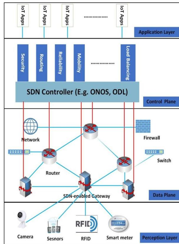
Fig. 2: SDN-IoT Architecture
