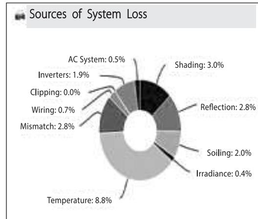
Fig. 7. Sources of system loss for 23.5-degree tilt angle
