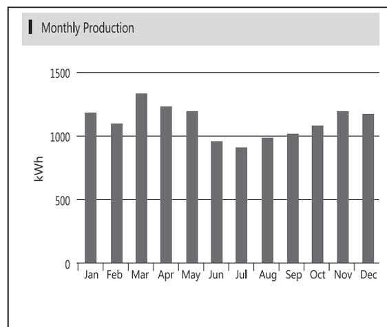
Fig. 2. Monthly Production of energy for tilt angle of 26 degrees
