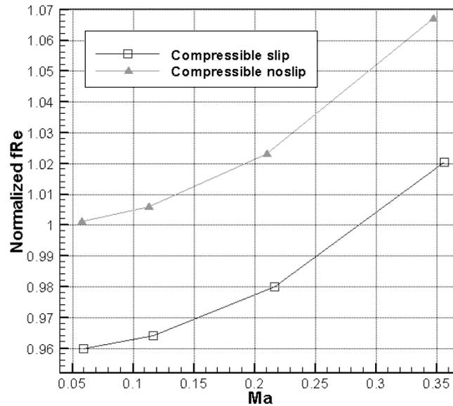
Fig. 8. The effect of average Mach number on friction constant at  $x/L = 0.9$ .
