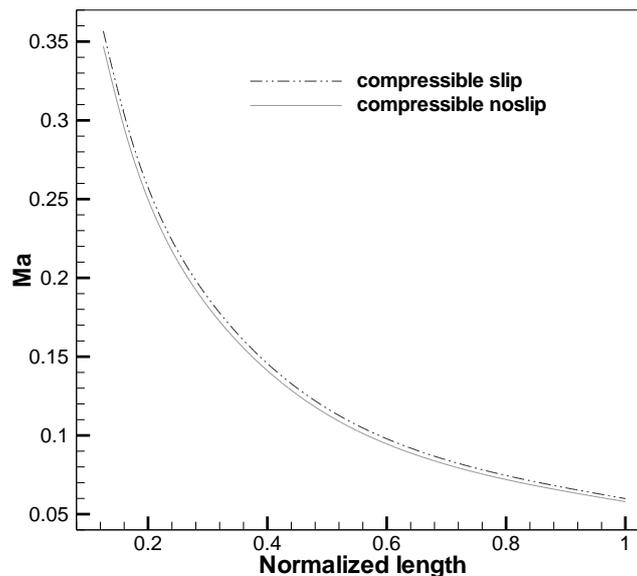
Fig. 9. The effect channel length on average Mach number at  $x/L = 0.9$ .
