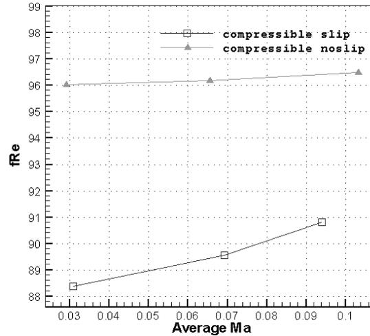
Fig. 5. The effect of average Mach number on friction constant at  $x/L = 0.9$
