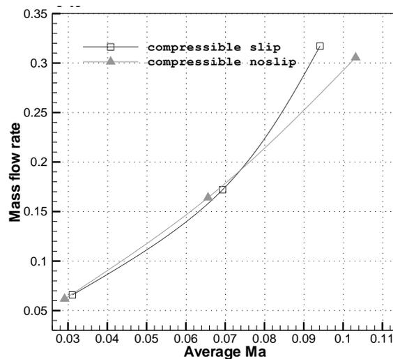
Fig. 6. The effect of average Mach number at  $x/L = 0.9$  on mass flow rate.
