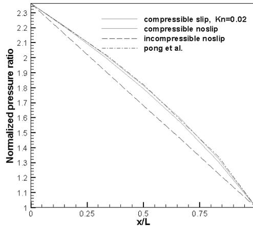
**Fig. 2.** Normalized pressure distribution along the centerline of the channel.
