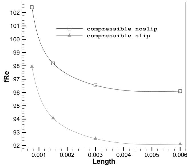
Fig. 7. The effect of channel length on friction constant at  $x/L = 0.9$ .
