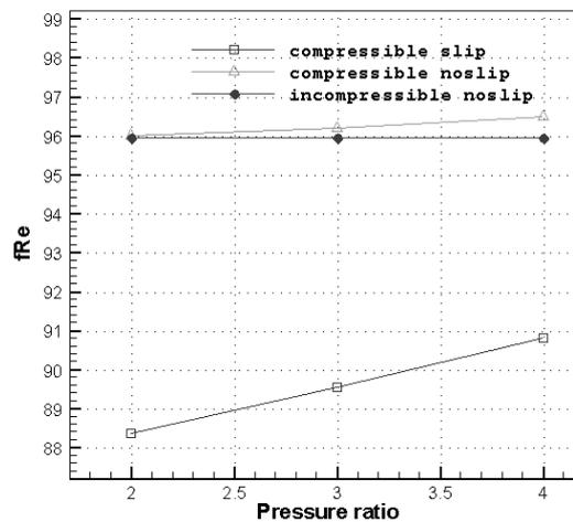
**Fig. 4.** The variation of friction constants at  $x/L = 0.9$  for different pressure ratios.
