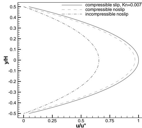
**Fig. 3.** Normalized velocity distribution on cross section at  $x/L = 0.9$ .
