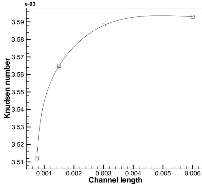
**Fig. 10.** The effect channel length on Knudsen number at  $x/L = 0.9$ .
