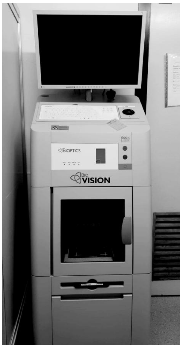
Figure 8: Mobile digital X-ray cabinet for assessment of radiological free margin of specimen per operatively
