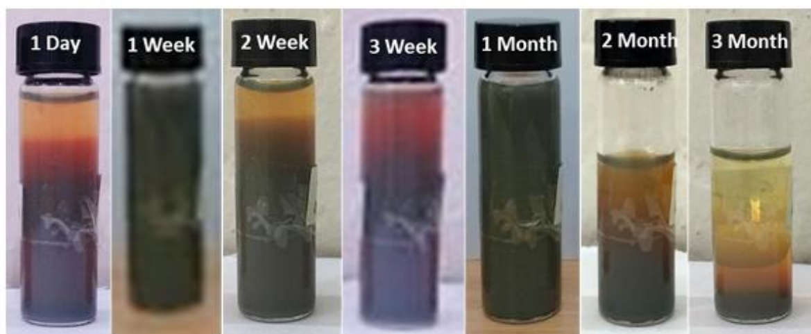
Fig. 6. Images of the TSC-capped AgNPs–water NFs at a concentration of 2.0 vol% prepared with the molar ratio of P:RA: CA=1:3:6 at different time intervals, observation of 1 day, 1 week, 2 weeks, 3 weeks, 1 month, 2 months, and 3 months.
