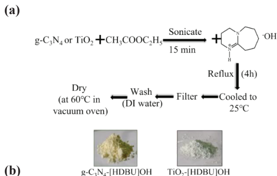
Scheme 2. (a) Schematic route for the preparation and (b) photographic images of g-C 3 N 4 -[HDBU]OH and TiO 2 -[HDBU]OH.
