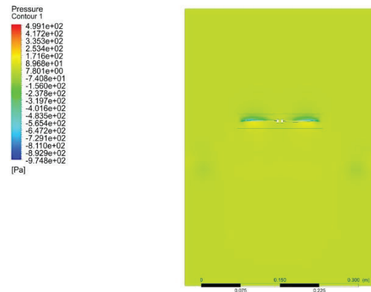
Fig. 13. Pressure Contour for RPM=8000.
