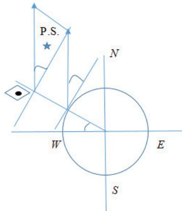
Fig. 2. Determination of Latitude
