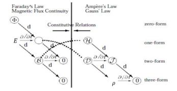
Fig. 3. Graphical representation of Maxwell's equation.
