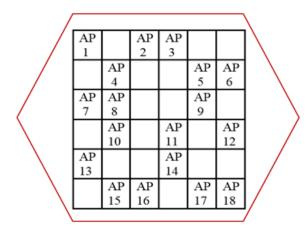
Fig. 2. WiMAX coverage areas with cells with and without WiFi AP
