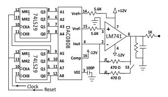
Fig. 5. Staircase voltage generator
