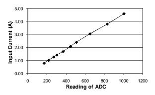
Fig. 11. Graph for calibration of current sensor
