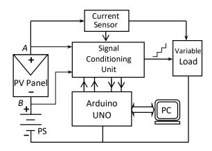
Fig. 1. Block diagram of the developed system
