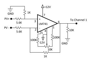
Fig. 2. Signal Conditioning Circuit for  $V_{PV}$
