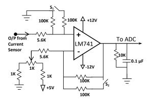
Fig. 3. Signal Conditioning Circuit for the Current Sensor
