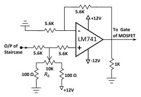
Fig. 7. Threshold voltage producing circuit
