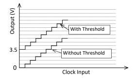
Fig. 8. Staircase voltage before and after using the Circuit of Fig. 7
