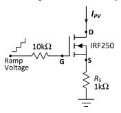
Fig. 4. Active load Circuit
