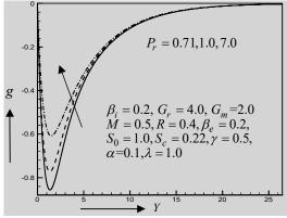
Fig. 6. Secondary velocity profile for different values of Prandtl number  $P_r$
