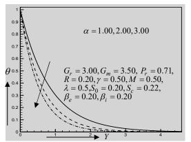
Fig. 16. Temperature profile for different values of heat source parameter  $\alpha$
