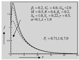
Fig. 5. Primary velocity profile for different values of Prandtl number  $P_r$
