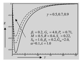
Fig. 9. Secondary velocity profile for different values of permeability  $\gamma$
