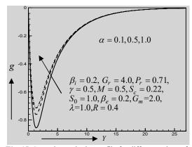
Fig. 15. Secondary velocity profile for different values of heat source parameter  $\alpha$
