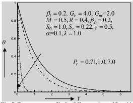
Fig. 7. Temperature profile for different values of Prandtl number  $P_r$
