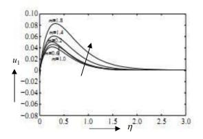
Fig. 20. Primary velocity profile of Maji et al.<sup>11</sup> for different values of Hall parameter m
