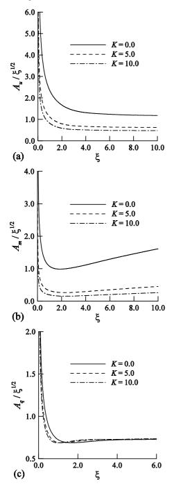
**Fig. 4.** Amplitudes of (a) skin friction, (b) couple stress and (c) heat transfer for different values of *K* while Ri = 2.0, Pr = 0.72 and M = 0.2.
