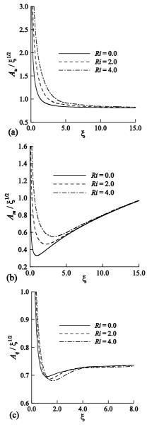
The effects of the Richardson's number, Ri, on the amplitudes of the skin friction, couple stress and heat transfer are shown in Figures 2(a), 2(b) and 2(c), respectively. From the figures, we observe that for higher Richardson's number, Ri, the amplitudes of skin friction and couple stress are higher. On the other hand, for Richardson's number, Ri, the amplitudes of heat transfer are higher near the leading edge while the reverse case is observed in the downstream region.
