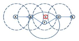
Fig. 2. New route possible using F
