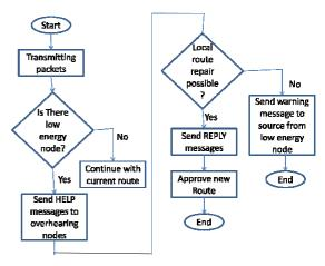
Fig. 11. Proposed route repair process
