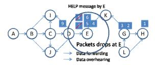
Fig. 13. Packets 7 and 8 are dropped at node E
