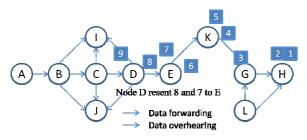
Fig. 15. Packets retransmission occurred
